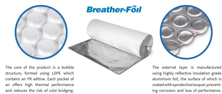
Our patented design effectivly allows timber frame constructions to breathe through the unique overlaping and venting method. Breather-Foil FR gives you a breathable and a high thermal efficent product with an over all thermal resistance value of 0.786 (m² K/W), equivalent to approximately 30mm EPS (expanded polystyrene) insulation.
