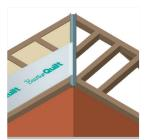
**7.1** Install the BreatherQuilt over the rafters, allowing the edge to drape over the valley gutter. Staple the product to the rafters, leaving the section over the valley loose.
