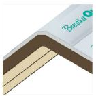
**5.2** Roll out BreatherQuilt over the ridge ensuring that a minimum 100mm overlap is maintained to the BreatherQuilt on both sides. Seal the joints using the horizontal jointing method (see section 2).
