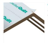
**6.1** Roll out the BreatherQuilt and fix in place using staples. Cut along the centre of the ridge beam and staple to the ridge beam to secure.
