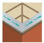
**8.2** On the other side of the roof, roll out the BreatherQuilt and butt-joint to the first piece.
