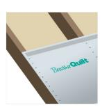
**2.1** Start at the bottom of the roof by rolling BreatherQuilt across the rafters and staple in place. BreatherQuilt features an easy to use built-in tape with easy peel backing.
