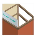
**8.1** Install the BreatherQuilt over the rafters, cutting the product to sit on the hip on the roof, and staple in place.
