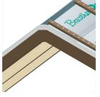
6.2 On the other side of the roof, roll out the BreatherQuilt and butt-joint to the first piece.
