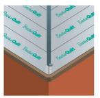
**8.3** Continue installing the product up the hip in the same fashion. Follow vertical joint detail (see section 1) and horizontal joint detail (see section 2), ensuring it is fully sealed.
