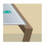
1.1 Unroll the BreatherQuilt over the top of the rafters. When you reach the end of the roll, cut the product so that it finishes in the middle of the last rafter, and staple in place.
