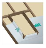
**4.3** Fold the flaps back up to the sides of the window and staple in place. Proceed with the next layer ensuring to follow the horizontal jointing detail.
