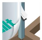
**7.2** Pull back the breather membrane on the product and carefully cut away the rest of the insulation, leaving just the grey membrane in the valley.
