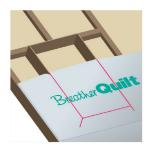
**4.1** Lay the BreatherQuilt over the window and cut out the section within the frame of the window (as detailed in drawing) on the top layer of BreatherQuilt only and fold this back.
