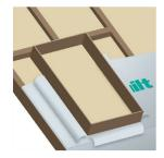
**4.2** Carefully cut and remove the rest of the material around the window's edge.
