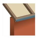
**3.1** Install a suitable eaves carrier over the rafters so that it runs down into the gutter (to manufacturers guidelines)
