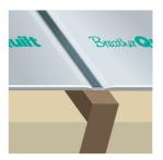
**1.3** Using the **ThermaSeal**<sup>™</sup> 50mm Waterproof Tape, tape over the joint and ensure it is fully sealed.
