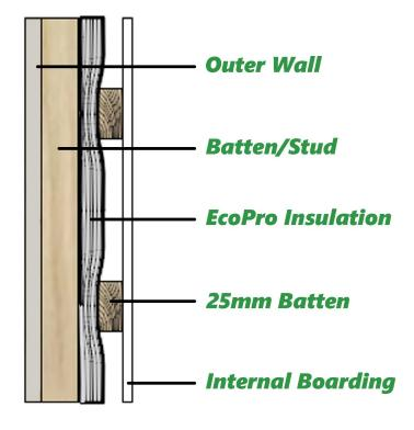
If Installing EcoPro onto the walls of your Static Caravan we would recommend the following;
